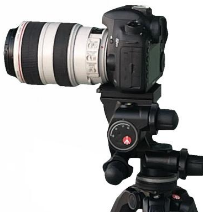
Fig.1-13 Lens installation completed
